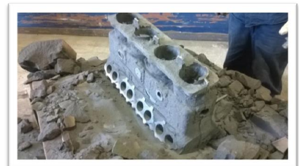
Trial casting emerging from destroyed sand mould.
