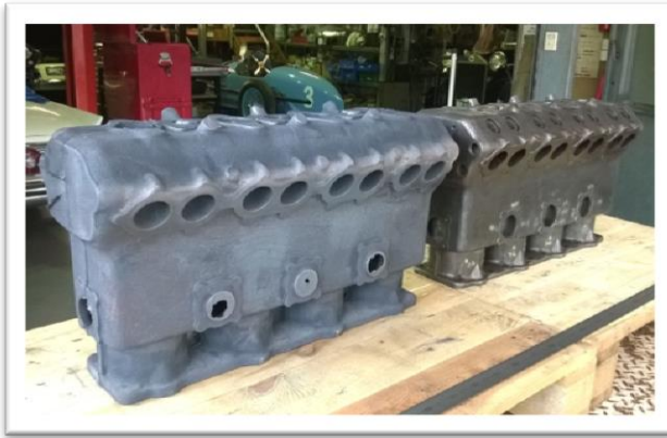
Trial casting (left) beside original engine block.
