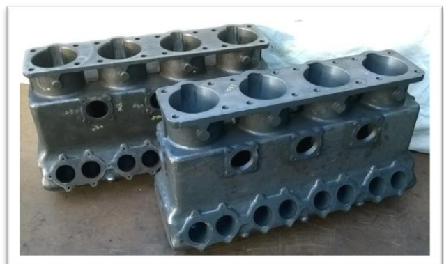
Production casting partly machined (with original).
