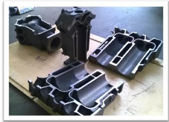
Trial casting sectioned for inspection and review.
