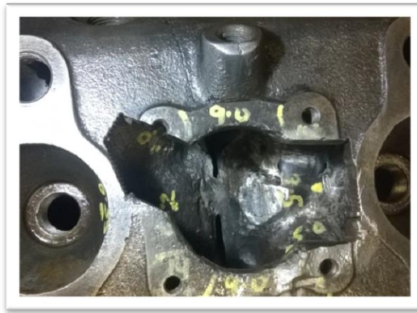
Casting failure No. 3 cylinder and area of failed repair.
