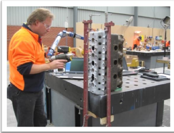
Laser scanning the engine block, 2015.
