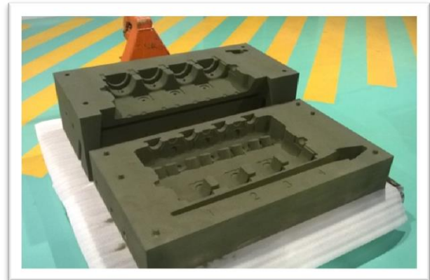
Sand printed main parts of the mould set.
