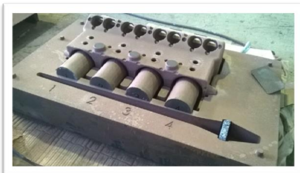
Sealed mould set, partly assembled.
