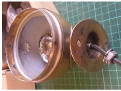
Fit and tighten the M8 nut and make a new rubber gasket.
