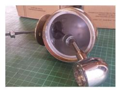
Open up centre hole in Rotax side light to 8mm. Fit washers under LED light to raise to centre line of Rotax.
